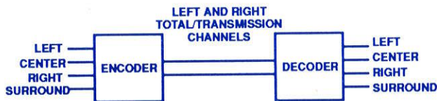
Fig. 2. Stereosurround Encoder/Decoder Block Diagram
