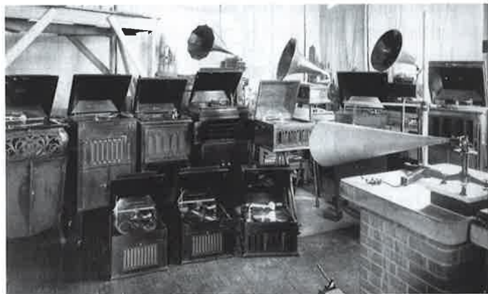
Figure 4. Dayton C. Miller was a consultant to Aeolian-Vocalion, a phonograph manufacturer. The photo shows the many types of phonographs that Miller measured and compared. On the brick pedestal (right front) is his calibrated Phonodeik with its conical horn. Photo ca. 1915. Courtesy of Arthur H. Benade, Case Western Reserve University, 1985.
